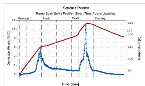
The Thermogravimetric Graph of solder paste during the reflow. The blue line represents evaporation of the paste. Most outgassing from the solder paste is in the beginning of the peak zones at the point where the solder starts to melt.
