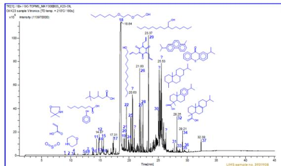
GC separation and Mass Spectrometry showed the chemical composition of the residues found in the first cooling zone.
